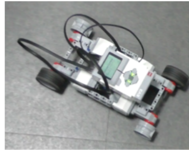
P2's Initial four wheel design that would not turn then the final four wheel design
