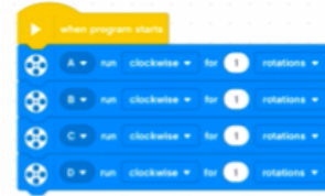
1. Sequentially coded run blocks to achieve forward motion.
