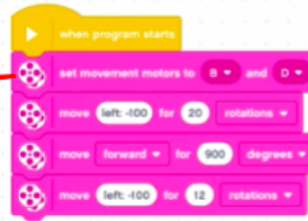
3. Final Solution code block controlling two motors on the two diagonal wheels.
