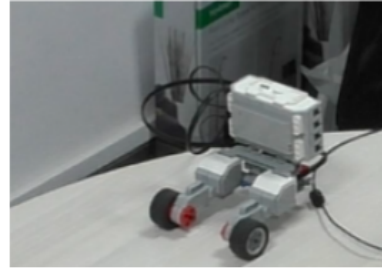
P1's Initial four wheel design that would not turn then the final caster wheel design
