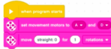
2. Parallely coded movement block controlling two motors but both coded to move straight
