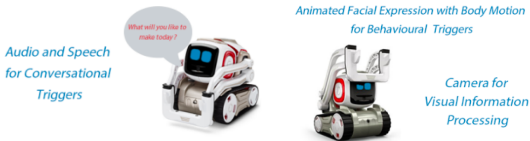
Figure C.4: Features of a physical pedagogical agent (COZMO) that would enable seamless interaction between TinkMate and the user.
