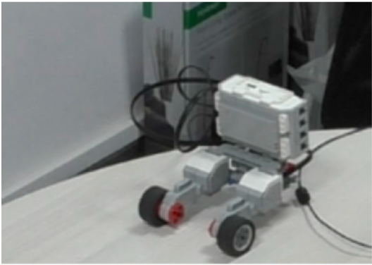
P1: Castor wheel based two motor solution
