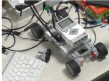
P2's Initial four wheel design that would not turn then the final four wheel design
