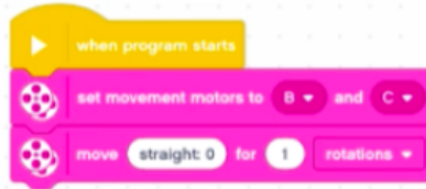
2. Parallely coded movement block controlling two motors but both coded to move straight
