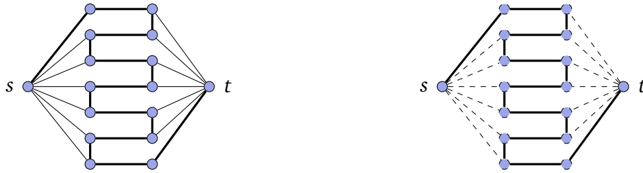
Figure 3.30: A weak counterexample for the max-flow problem. A flow of O(n) units exists but the weak algorithm finds a flow of only 1 unit.
