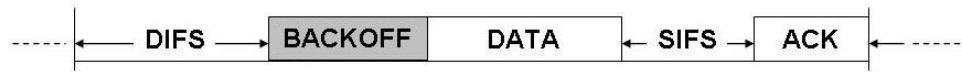
Figure 4.1: DCF mechanism: Timing diagram for events during data transfer between two nodes in the 802.11 DCF MAC protocol .
