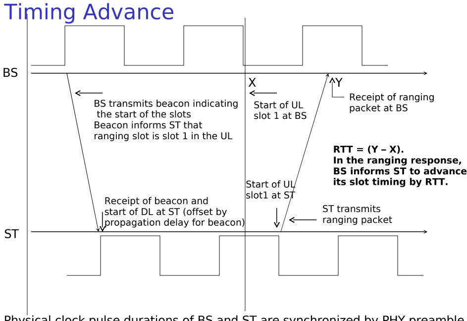
Physical clock pulse durations of BS and ST are synchronized by PHY preamble  $^{24}_{24}$
