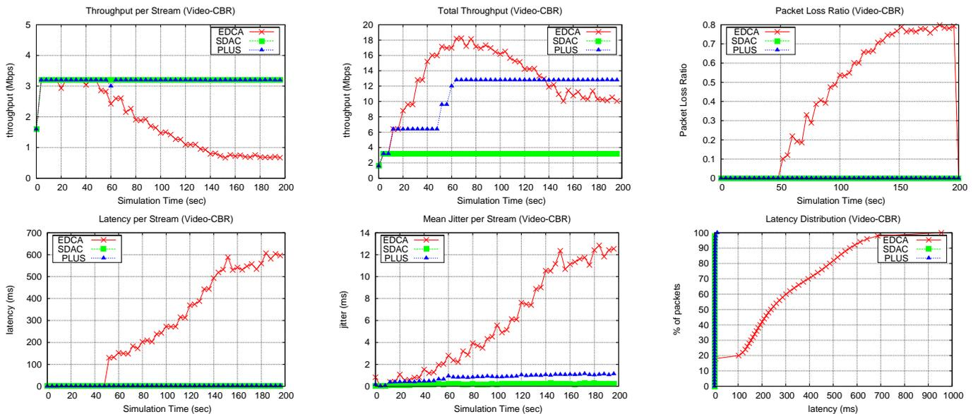
Fig. 5. CBR throughput and latency characteristics
