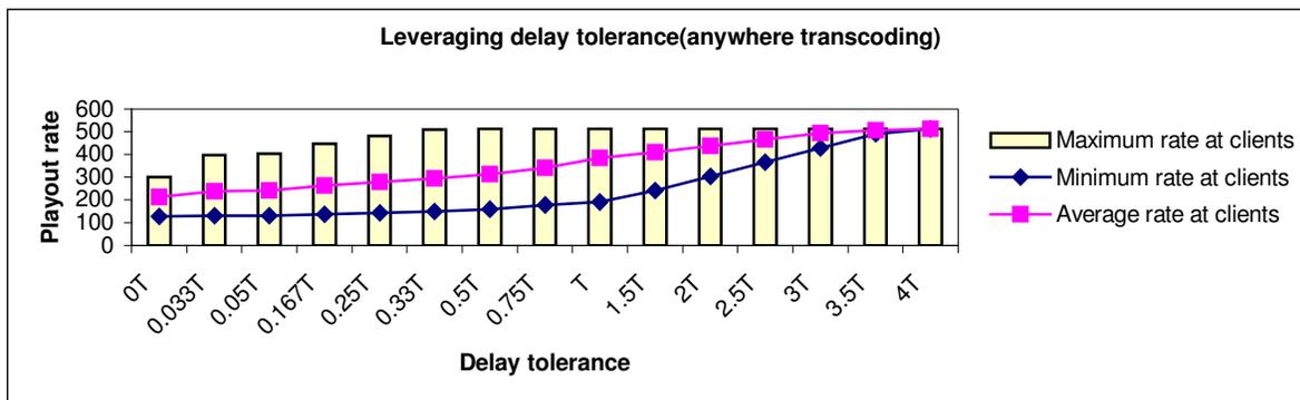
Figure 3: Improved quality through exploiting client delay tolerance
